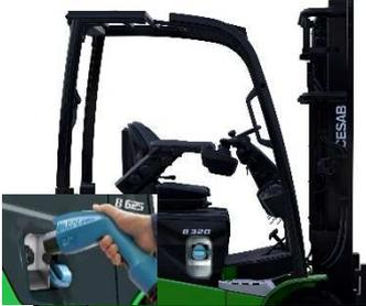
The Li-ION charging port is mounted on the side panel so connecting is effortless!
