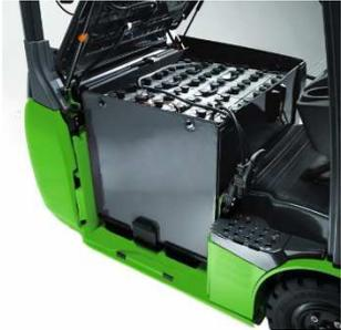
For applications where lead-acid batteries are used, batteries can be swapped in minutes thanks to the optional sideways battery extraction.
